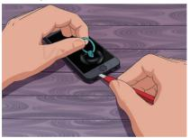
O2 Secure a suction cup to the front of the phone. Press the suction cup onto the screen, just a bit above the Home Button. Apply enough pressure to form a tight seal. A tight seal is necessary to hold this front half up as you try to disconnect it from the bottom.
