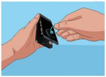
05 Open the iPhone so that the display is at a 90° angle to the base. Use the top as a hinge, and rest the screen against a book or a box at a 90° angle so that you can work on the insides without holding it. Don't let it open further, or you may damage the cables connecting it.
