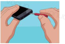
01 Remove the two Pentalobe screws next to the Lightning port. This is the charging port at the bottom of the phone. You'll need a Pentalobe screwdriver to remove these screws.
