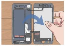
11 Open the display to the right. It should fold open like a book, with the interior of the iPhone now exposed and the still-connected display and screen face-down to the right of the case.
