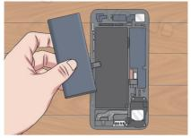
28 Remove your iPhone's battery. At this point, you can place a new battery in the iPhone, or let the phone dry as needed if it has suffered water damage.
