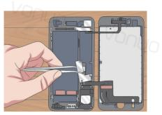
13 Remove the display bracket and set it aside. You'll see two black strips of plastic beneath it: one running parallel to the battery, and one running perpendicular.
