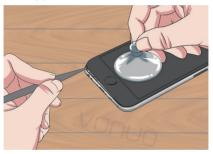
08 Lift the screen up to form a ten-degree angle with the phone's case. Lifting the screen any higher than this will break the fragile display cables, so proceed with caution on the side when doing this.
