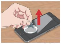
05 Pull up on the suction cup to lift the screen. The screen should only lift a fraction of an inch away from the case. Pulling too hard may rip the display from the case, so be gentle. Hold the rest of the iPhone down with your other hand while you pull the suction cup. If the screen won't come up, try heating the bottom of the iPhone for another few minutes.
