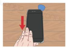
10 Pull the screen down toward the bottom of the phone. You should only have to pull it a few millimeters down to clear the plastic clips at the top of the iPhone
