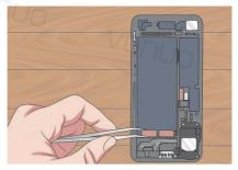
25 Peel back the three adhesive strips from the bottom of the battery. You'll want to use a pair of needle-nose pliers or tweezers for this step.
