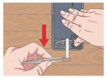
27 Pull the other two strips out. Make sure you're holding down the battery while pulling out the last one so that the battery doesn't get ejected from the iPhone's interior.
