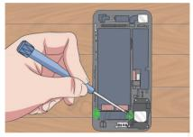
23 Remove the three Phillips screws from the Taptic Engine. All three of these screws are 1.5 millimeter screws.
