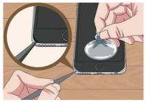
06 Insert your spudger into the space in the lower-left corner of the iPhone. There should be a space created by gently pulling up on the suction cup, and your spudger should fit snugly into the gap. Make sure you're using a plastic spudger and not a metal one, as a metal spudger will damage your phone.
