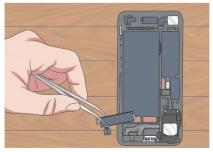
24 Lift gently the Taptic Engine out of the case. With the Taptic Engine out of the way, you're finally ready to remove the iPhone's battery.
