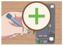
20 Remove the two Phillips (+) screws from the barometric vent. This black bracket is in the bottom-left corner of the iPhone's case. You'll find a 2.9 millimeter screw and a 2.1 millimeter screw holding it down.
