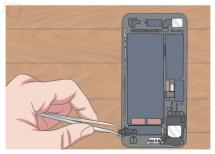
21 Remove the barometric vent. You should now be looking at the Taptic Engine's connector, which is a black piece of plastic like the rest of the connectors you've unattached so far.
