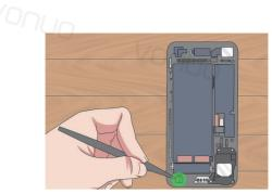
22 Pry up the Taptic Engine's connector with your spudger. Doing so will disconnect the Taptic Engine from your iPhone's logic board, which will in turn allow you to remove the Taptic Engine.
