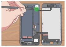
18 Use the spudger to pry up the connector. Doing so will remove the second display ribbon from the iPhone's interior.
