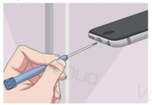
02 Remove the Pentalobe screws from each side of the Lightning port. The Lightning port is at the bottom of the phone. You'll need a 3.4 millimeter Pentalobe screwdriver to remove the two screws here.
