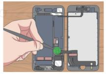
15 Use the spudger to lift up the parallel plastic strip and the grey strip beneath it. Doing so will detach the ribbon here from the iPhone's interior, thereby disconnecting one of the two display ribbons.
