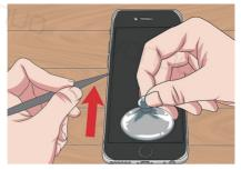
O7 Slide the spudger up the left side, then repeat on the right side. Twisting the spudger back and forth should gently pry the screen away from the phone's casing. Do not use the spudger near the top of the phone—there are plastic clips that hold the top of the screen in place, and doing so will break them. Instead, only move the spudger about halfway up each side.
