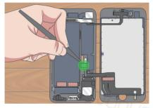
14 Use the spudger to lift up the perpendicular plastic strip. This strip is the battery connector; detaching it will disconnect the display from your iPhone's battery.
