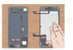
19 Set the iPhone's display assembly aside. It should be completely removed at this point.
